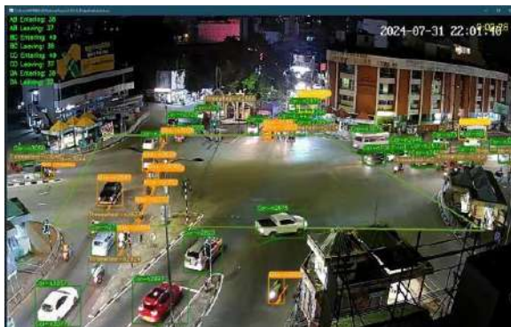
Fig. 8. Processed frame from YOLO model
